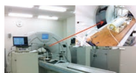
Visualization of CO 2 distribution in a sample rock using X-ray CT
