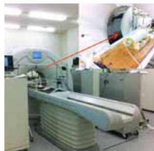
Visualization of CO 2 distribution in a sample rock using X-ray CT
