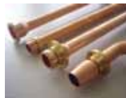
Technology to process the ends of copper pipes
